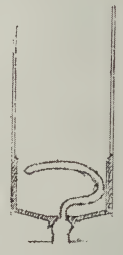
Fig. 4. End view of one of the hollow rods, full size. Showing bearing on rod which takes the thrust of wheel.
